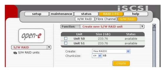
After clicking "create" button, the status will change to "in use" with additional information describing the kind of a disk array (e.g. MD0 is RAID 1)
